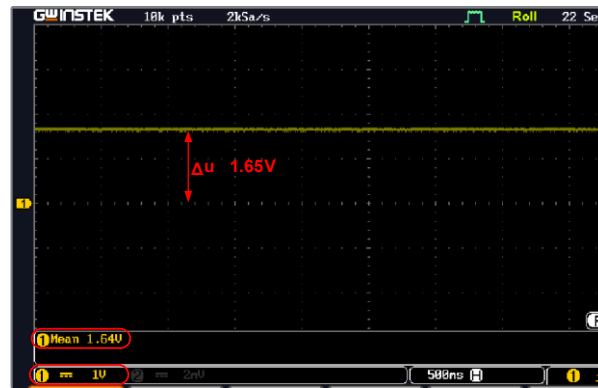
Figure 5. The output voltage of the INA241A2 amplifier in the absence of input voltage (amplifier supply voltage V_s = 3.3 V).
